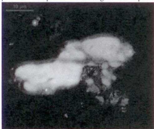
Fig.1. Confocal scanning laser microscopy optical slice through the center of a solid OMA. The signal emitted in the green channel represents the fluorescent oil. The signal in the red channel is the reflectance from mineral particles.
