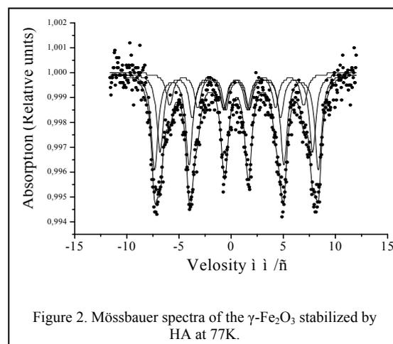
Figure 2. Mössbauer spectra of the  $\gamma$ -Fe<sub>2</sub>O<sub>3</sub> stabilized by HA at 77K.
