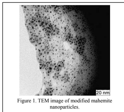
Figure 1. TEM image of modified mahemite nanoparticles.
