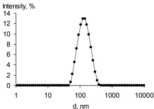
Figure.1 Particles size distribution for magnetic nanoparticles obtained at  $650^\circ\text{C}$  and stabilized by HA as measured by dynamic light scattering (DLS); ( $D=145\pm 60$  nm).
