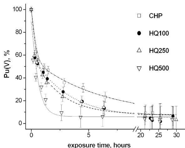
Fig. 2. Pu(V) reduction by hydroquinone-enriched humic derivatives under anoxic conditions at neutral pH ( $7.5 \pm 0.2$ ):  $C_{\text{tot}}(\text{Pu}) = 2.3 \times 10^{-9}$  M,  $C_{\text{tot}}(\text{HS}) = 10$  mg/L,  $I = 0$  M.
