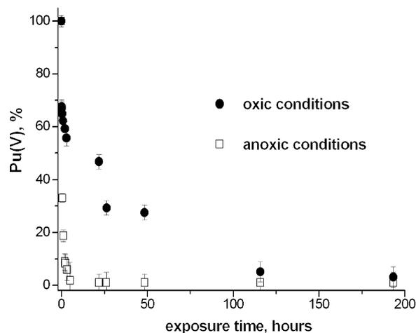
Fig. 1. Pu(V) reduction by leonardite HA (CHP) under oxidic and anoxic conditions:  $C_{\text{tot}}(\text{Pu}) = 7.17 \times 10^{-9}$  M,  $C_{\text{tot}}(\text{HS}) = 10$  mg/L,  $pH 4.7 \pm 0.2$ ,  $I = 0$  M.
