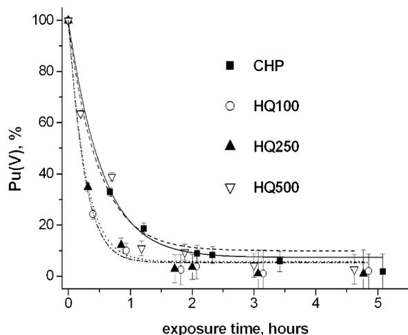
Fig. 3. Pu(V) reduction by hydroquinone-enriched derivatives under anoxic conditions at acidic pH ( $4.5 \pm 0.2$ ):  $C_{\text{tot}}(\text{Pu}) = 2.3 \times 10^{-9}$  M,  $C_{\text{tot}}(\text{HS}) = 10$  mg/L,  $I = 0$  M.
