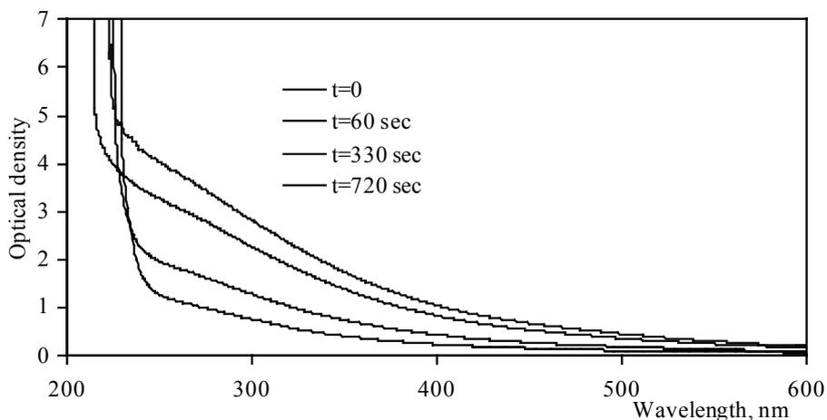
Figure 4. UV/Vis-spectra of CHP-K in the course of ozonation (pH=5.5).
